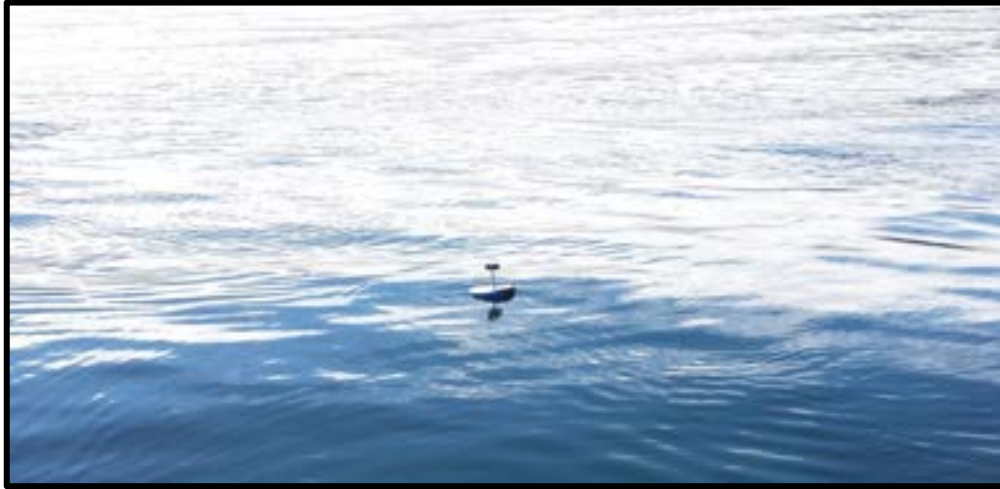
Figure 3. GPS surface current tracking buoy developed by the Institute of Ocean Sciences. To minimize the direct effects of weather on the SCT movement, most of the SCT floats below the surface with only the SPOT Trace above the water surface.
