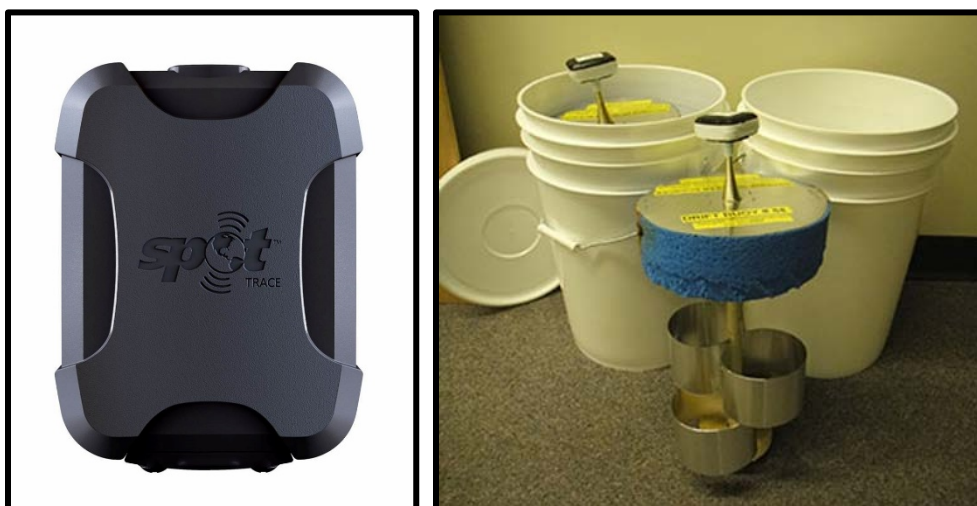
Figure 2a,b. Surface current tracker (SCT) buoy. The SPOT Trace™ device (a) is screwed to a spring which is then attached to the drifter (b).
