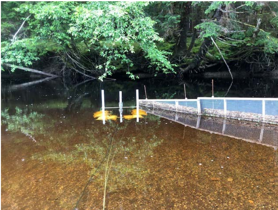
Photo 5 – Sonar and mounting frame
