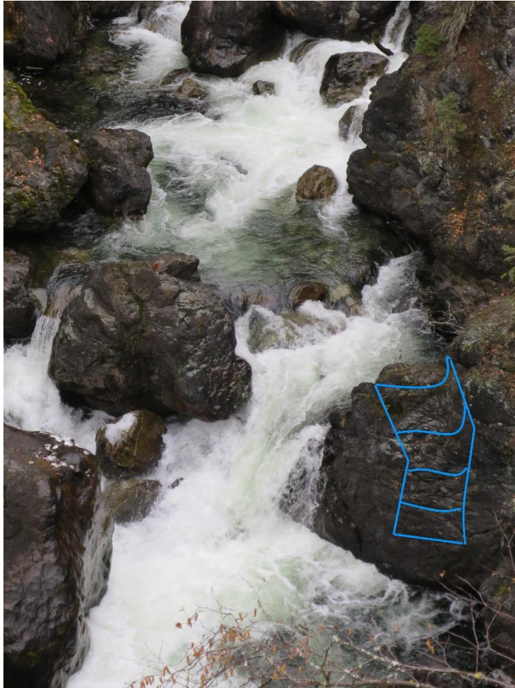
Photo 10: A conceptual design configuration for the rock notch design option.
