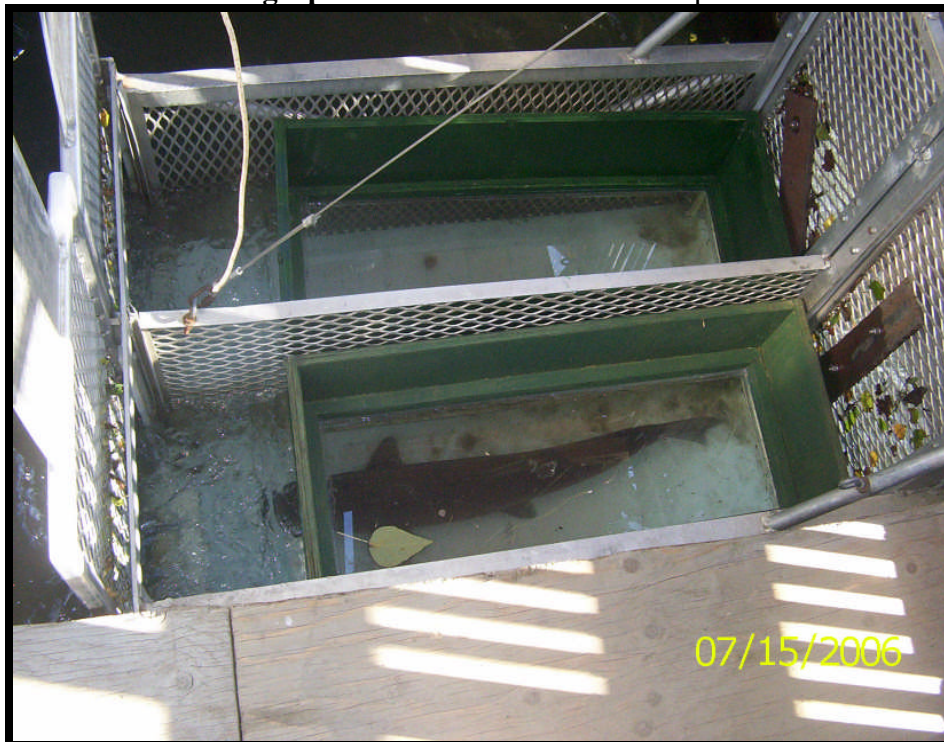
Photograph 5. Plexiglass viewing box used to identify fish as they swim through traps.
