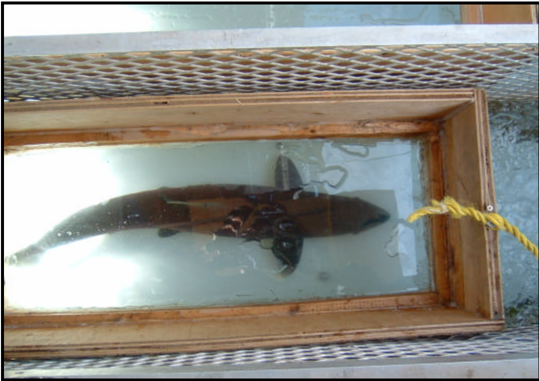
Photograph 5. Plexiglass viewing box used to identify fish species as they swim through trap boxes.
