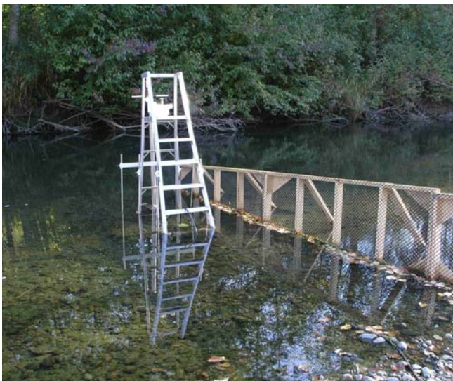
Figure 3. DIDSON ladder and diversion weir
