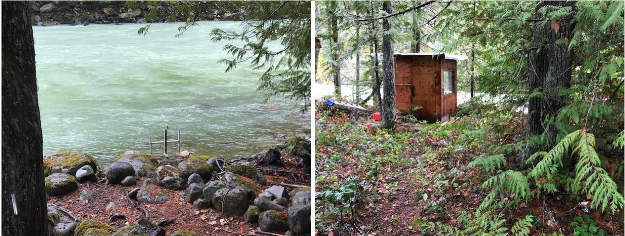
Figure 2. Photographs of the H-mount used to deploy the ARIS 1200 in the Lillooet River just below the mouth of Rogers Creek (left) and the portable shed used to house the batteries and electronic components used to operate the ARIS system (right).
