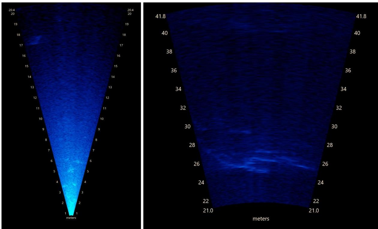
Figure 3. Screen shots taken of still ARIS imagery showing the FOV for the near-field zone (left) and far-field zone (right). Brighter features within the fields-of-view represent cobble and boulder substrate.
