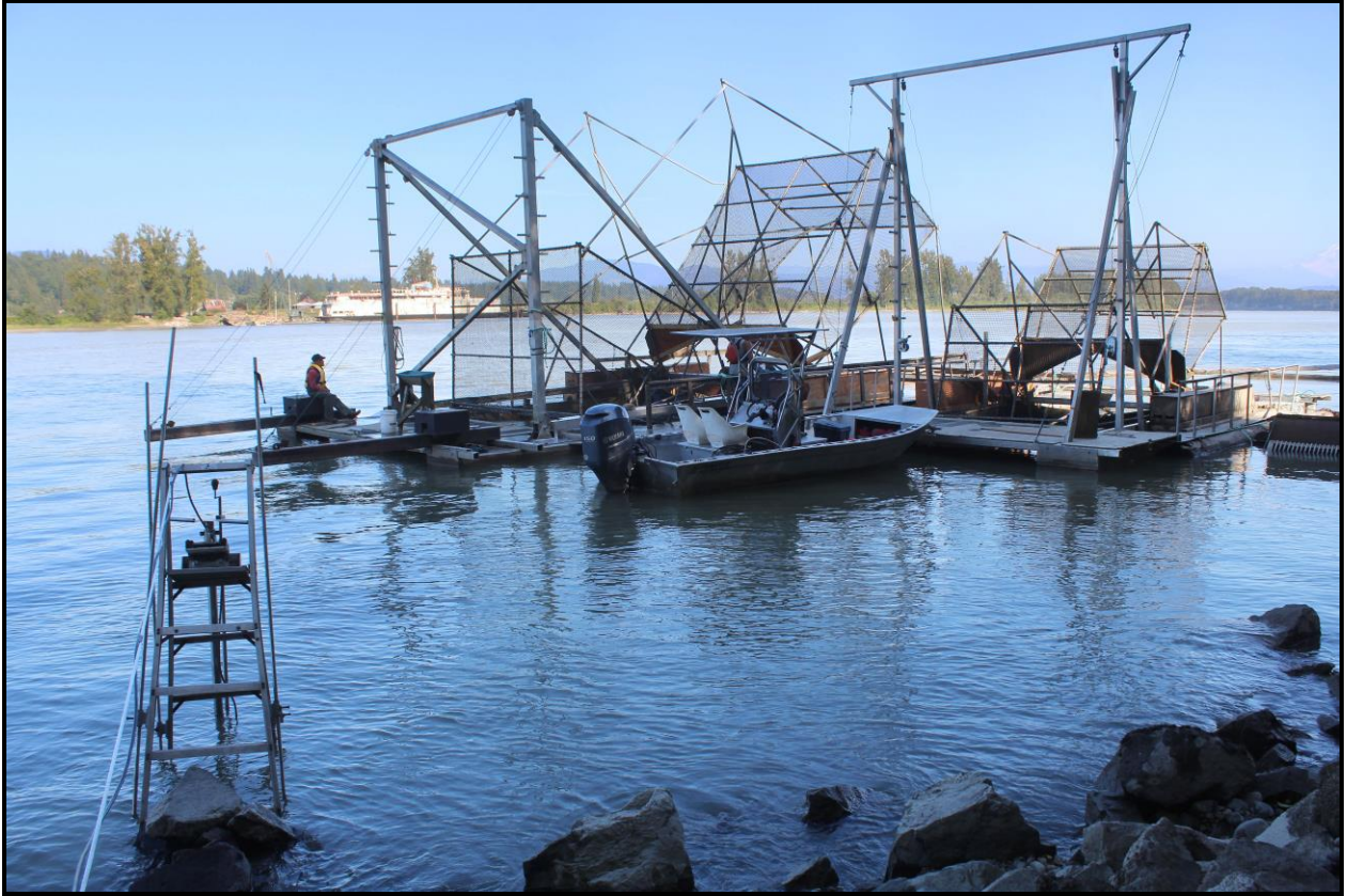
Figure 2. Fishwheel and sonar setup in 2019. Sonar on ladder mount near shore, small fishwheel on inside and large fishwheel on outside.
