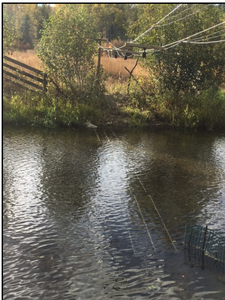
Figure 2: Resistivity counter installed in Bessette Creek, BC.
