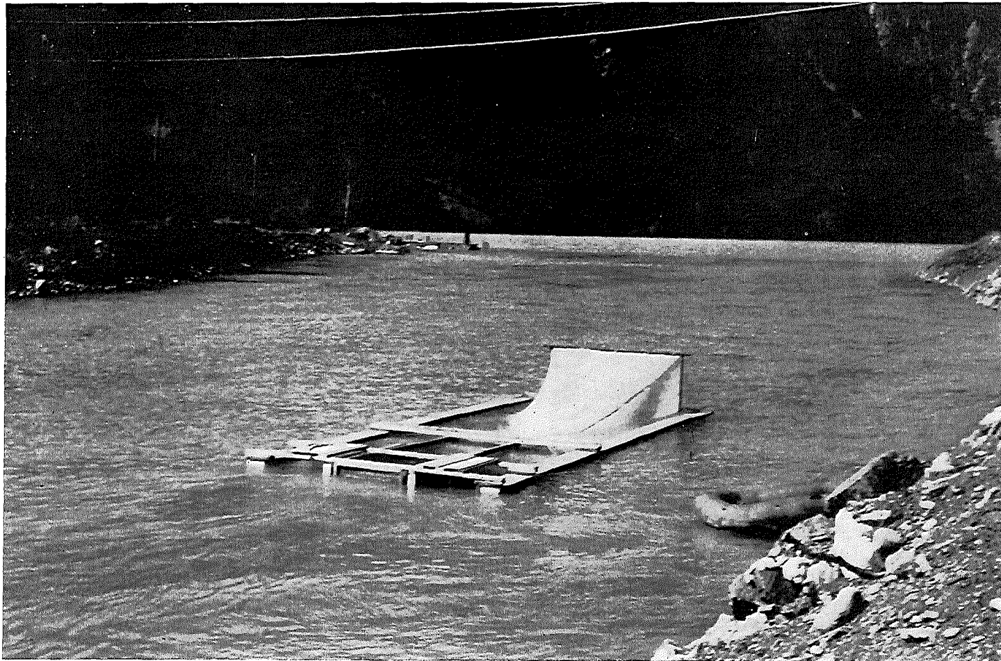
Fish and power research at the Seton Creek hydroelectric station. The fyke net shown is being used to determine the rate of passage of sockeye migrants through the fourteen mile length of Seton Lake.
