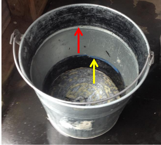
Figure 12. The volumetric “calibration” bucket used to quantify smolt numbers. The lower yellow arrow indicates the full mark to which water is added prior to filling with smolts. The upper red arrow indicates the level indicating the full mark to which smolts are added. As soon as the smolt “full” mark is reached, the live smolts are immediately transferred to the counting shed ( Figure 14 ) where smolts are examined for tags.
