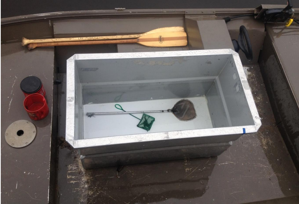
Figure 11. View of the metal tank used to transport over 3,000 tagged sockeye smolts to the release area of Nilkitkwa Lake, 6 to 8 km upstream. Fresh river water was pumped into the tank at the smolt trap until approximately half full. One or two battery-powered aerators aerated the tank water until all smolts had been released.
