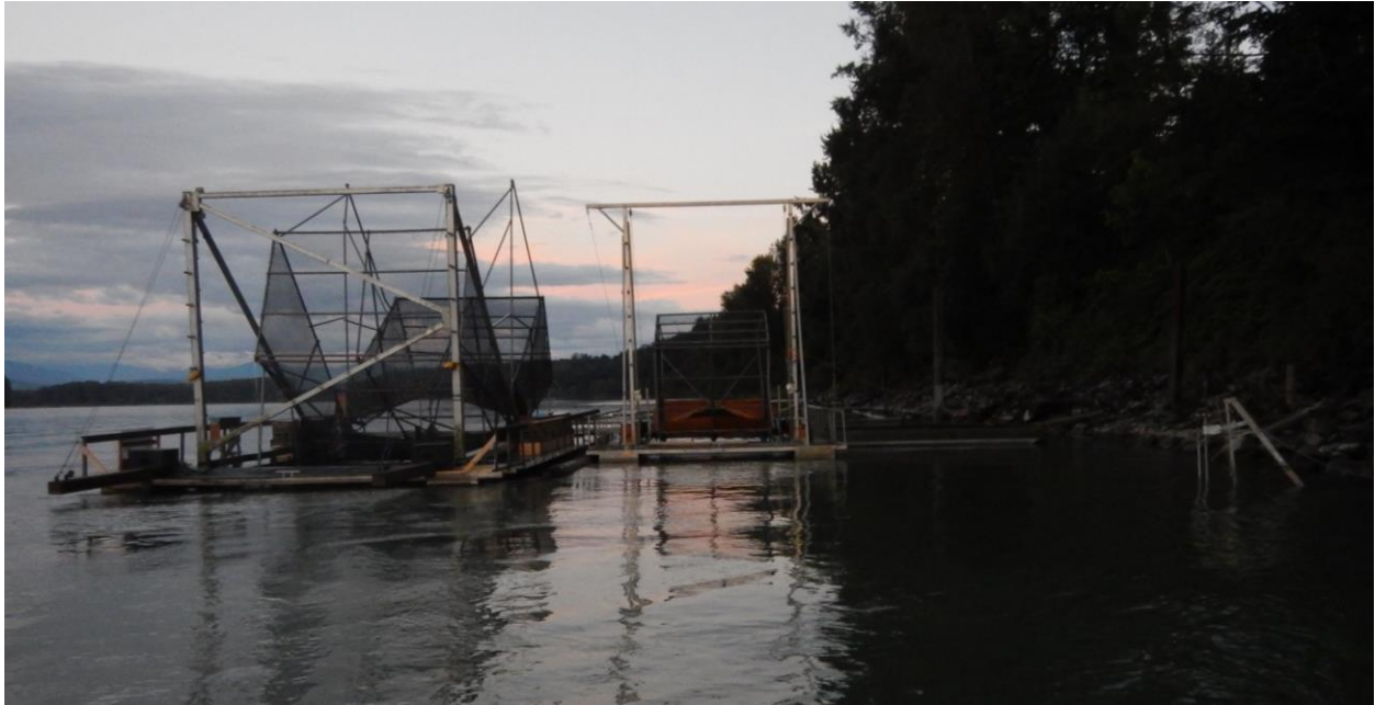
Figure 2. Fishwheel and sonar setup in 2017. Sonar on ladder mount near shore, small fishwheel on inside and large fishwheel on outside.
