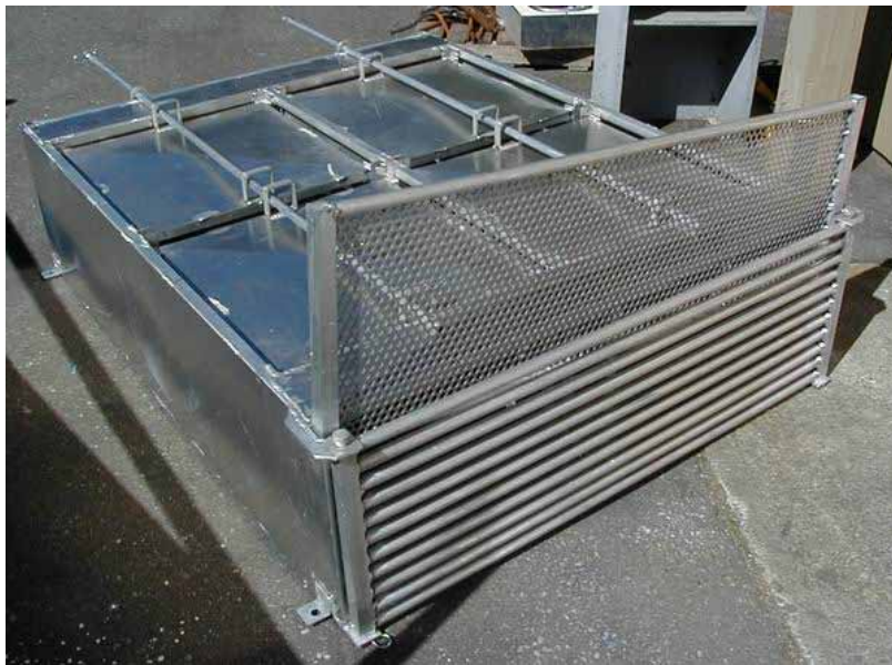
Figure 3. Screen modification for high velocity events – prior to final lid design (see Fig 2)
