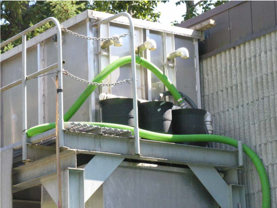
Figure 30. Close-up of black aeration pots for tanks 5 and 6 at Puntledge Lower site.
