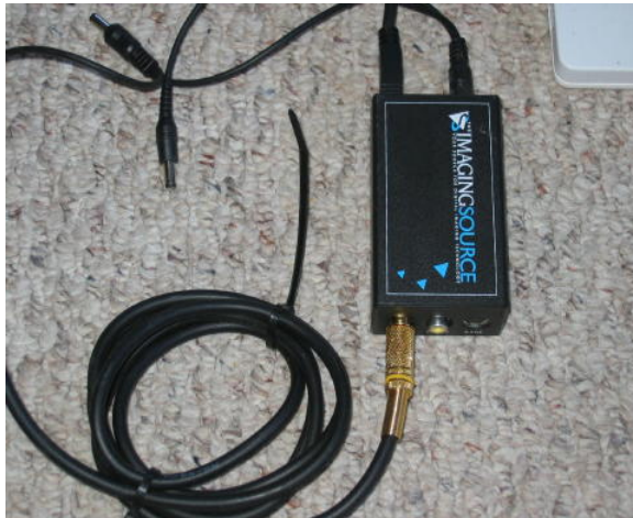
Analog to Digital Convertor with Fire wire cable (bottom of photo)
