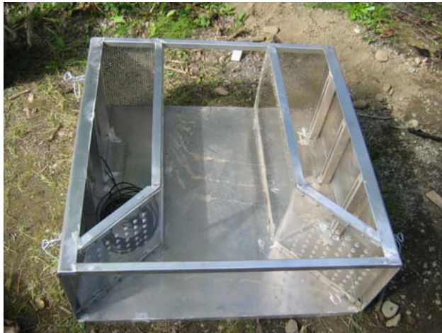
Underwater Camera Box (salmon swim through box from bottom to top of photo). Cameras can be mounted on either side of the box protected by internal plexiglass walls
