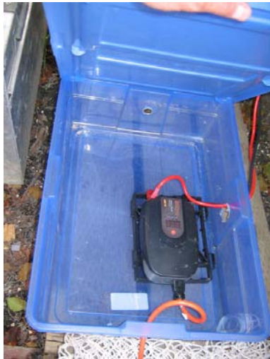
Power Invertor (400 watts). Converted 12 volt battery power to 110 volts.
