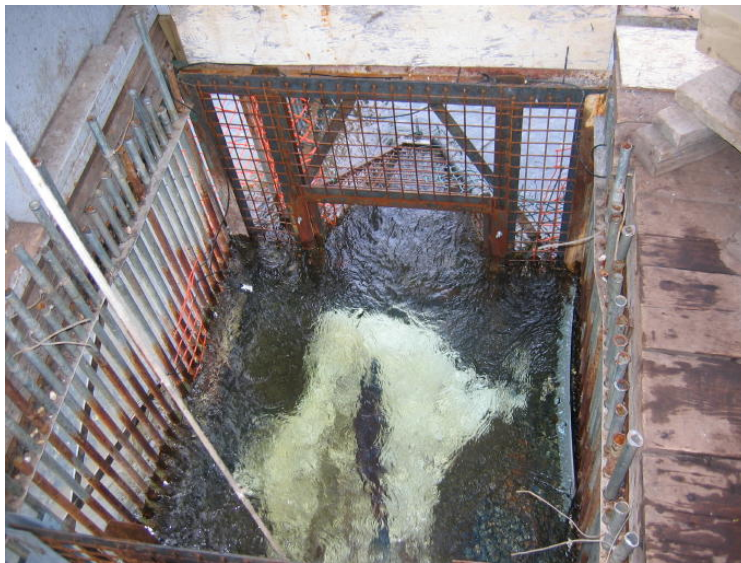
Weir passage chamber where cameras were mounted to record salmon migration. Note salmon heading upstream.
