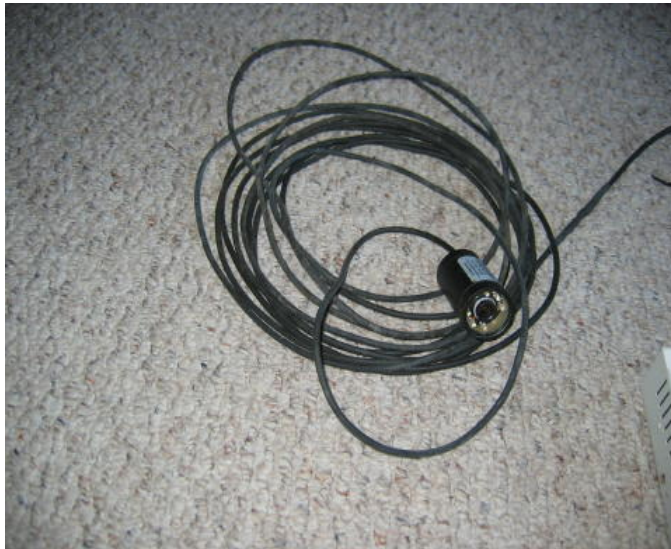
Underwater video camera with cable. Note LED lights around the camera lens
