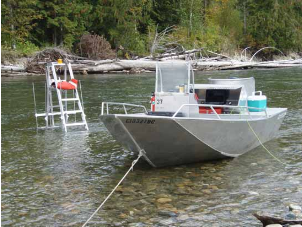
Photo 1. View of the ProViewer hydroacoustic site on the Adams River. The in stream step-ladder, with the adjustable pole mount and attached sonar head, was also used as a tower for visual counting. The boat anchored to the shoreline housed the operating computer and junction box with cable attached to the sonar head. Photo taken by Ted Sweeten on October 4, 2007.
