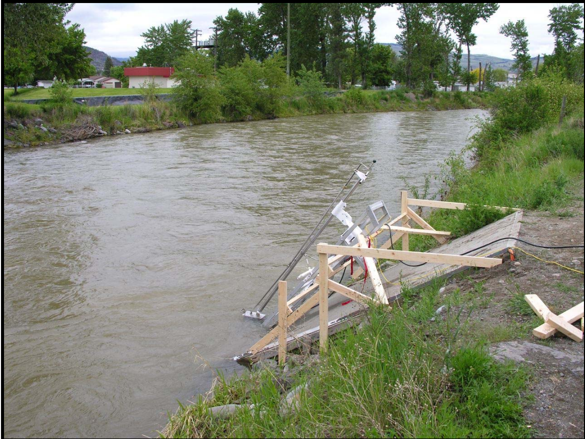
Figure 1: Set up for DIDSON unit. Aluminum, adjustable mounting apparatus of DIDSON unit was secured to fabricated 2x4 framework with screws and ratchet straps. A backup rope was tied to the DIDSON unit and secured to a large tree.
