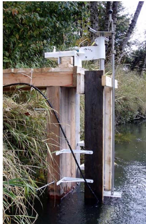
Figure 4. High water redeployment of DIDSON unit to bulkhead.
