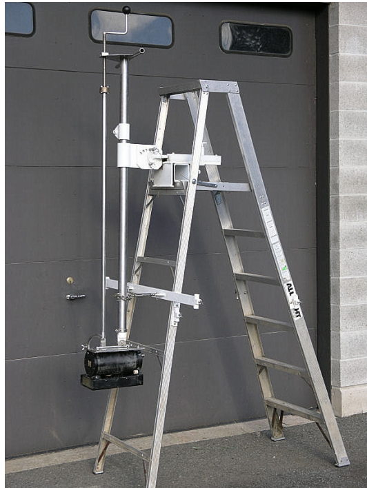
Figure 2. DIDSON ladder mount
