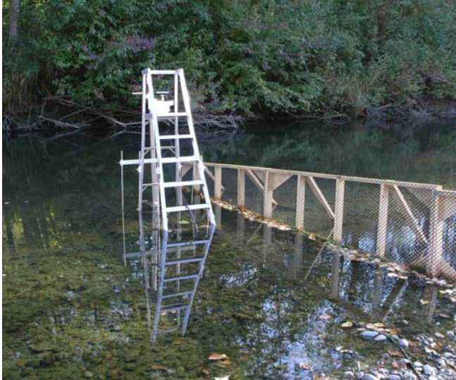
Figure 3. DIDSON ladder and diversion weir
