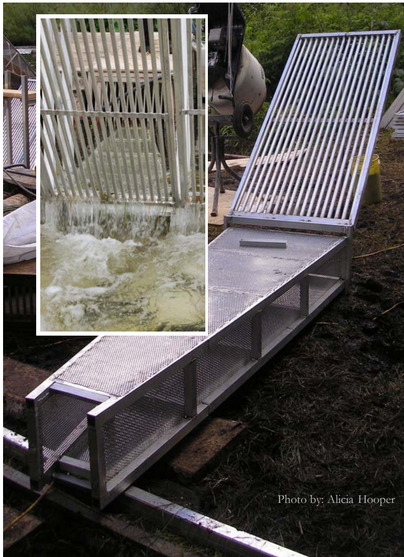
Figure 9. Aluminum opening inserted into panel frame to create the fence entrance. The narrow end (bottom left) inserts into a live box.
