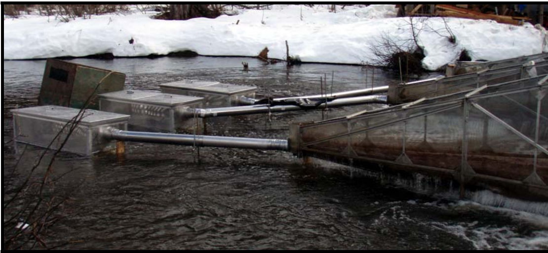
Figure 4. Smolt system assembled May 7th with three separate capture units.
