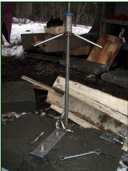
Figure 3. Screw jack mechanism to adjust downstream trap height.
