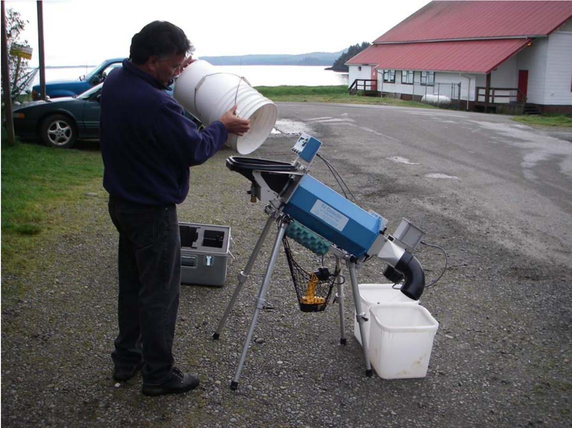
Figure 1 Haida Fisheries technician testing T4 CWT Tunnel Detector prior to deployment at Deena Creek field site.
