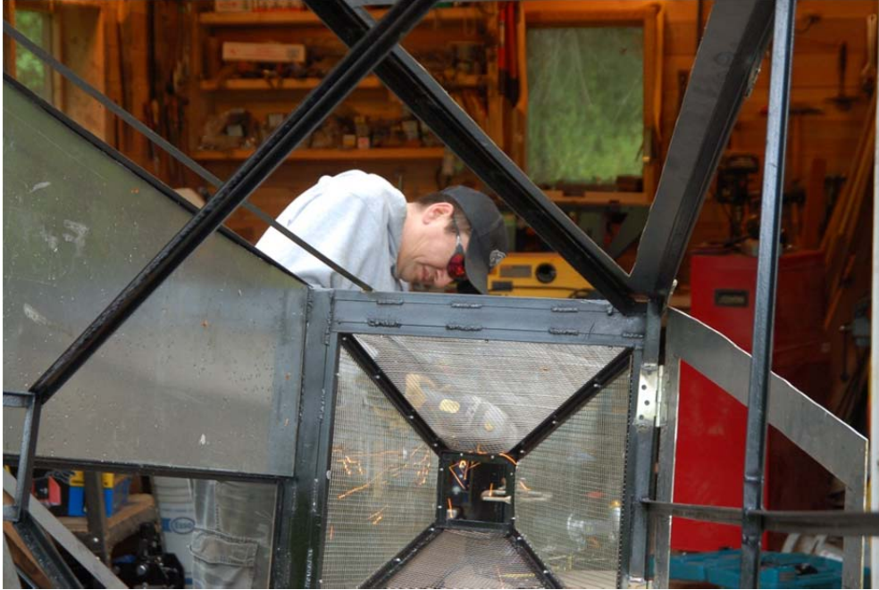
Figure 4. Fabrication of mesh covering to fyke frame of smolt trap #2. The trap bottom is to the left (half covered).
