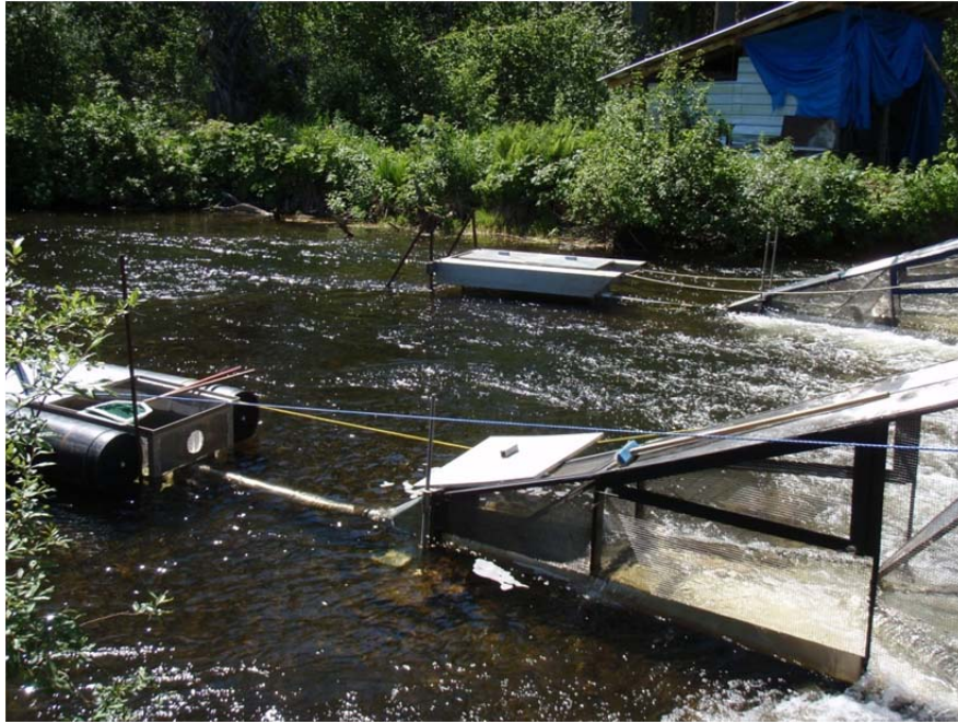
Figure 6. Smolt fyke traps and outlets leading to floating live boxes which are secured by steel rods (newly constructed trap #2 in foreground).
