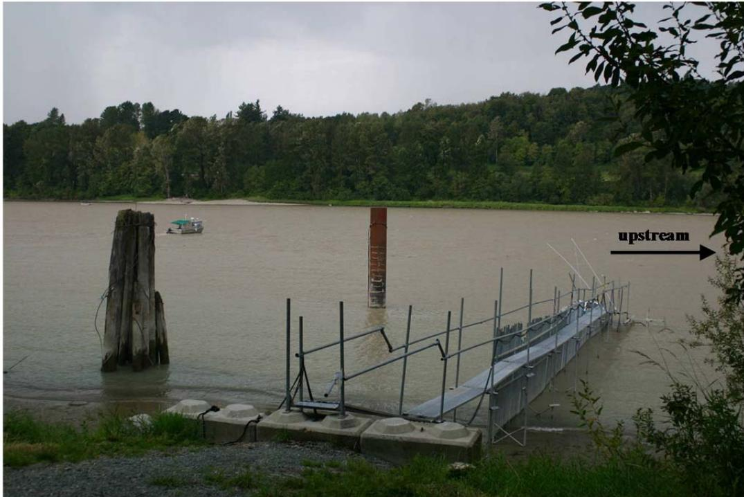
**Figure 3.** A left-bank view of the PSC Mission hydroacoustic site. The iron dolphin, located at 49°08.175'N; 122°16.466'W, is the geographic reference for positioning all sampling apparatus for the field program at the site. Also shown are the mobile survey vessel and a fish-deflection weir (approximately 35 metres in length) on the left bank. The weir prevents fish from swimming behind the shore-based sonar beams.
