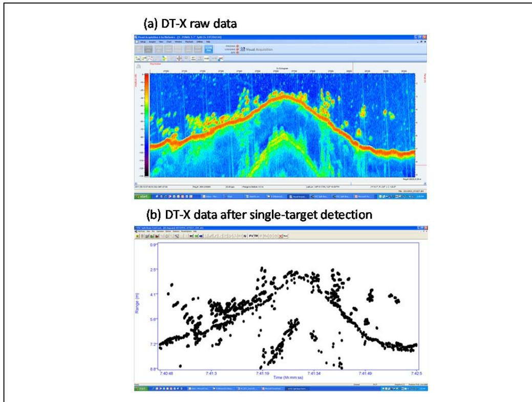
**Figure 6.** (a) DT-X split-beam raw data vs. (a) after single-target detection using criteria shown in Fig. 5. Data source: 20110910\_071827.
