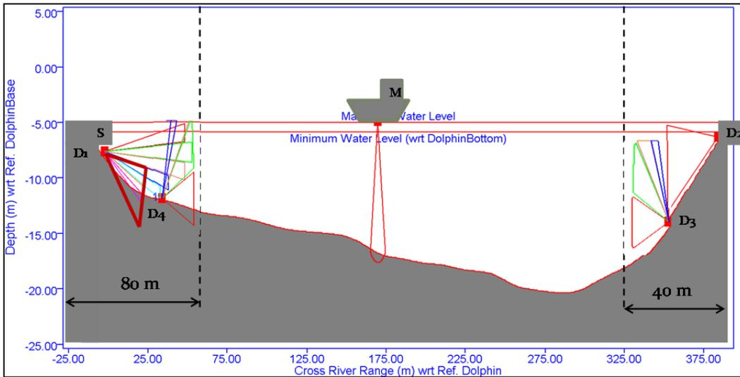
**Figure 1.** Deployment locations and sampling geometry of left-bank (S) and mobile (M) split-beam systems and 4 DIDSON imaging sonar units (D1, D2, D3, D4). The 6 sonar systems formed the proposed estimator.
