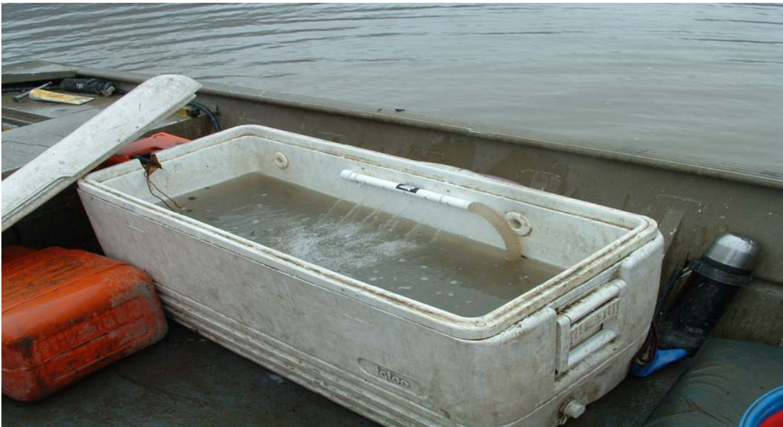
Appendix Figure 4. Aerial tank used to transport Stikine River Chinook and coho smolts to the tagging site located near the DFO camp.
