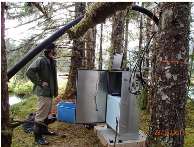
**Figure 1 Video creel system. Solar charging components, batteries and DVR enclosed in an aluminum weather proof box that is bolted to a concrete pad.**
