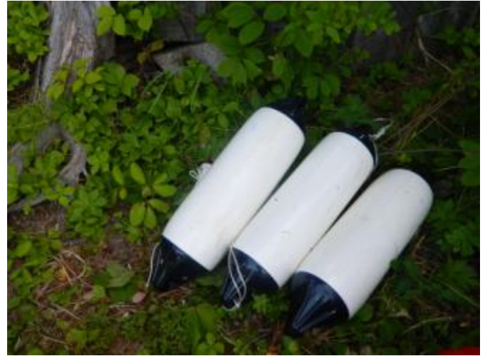
Figure 6. 8.5" x 48" Fender floats used along outer edge of main dock
