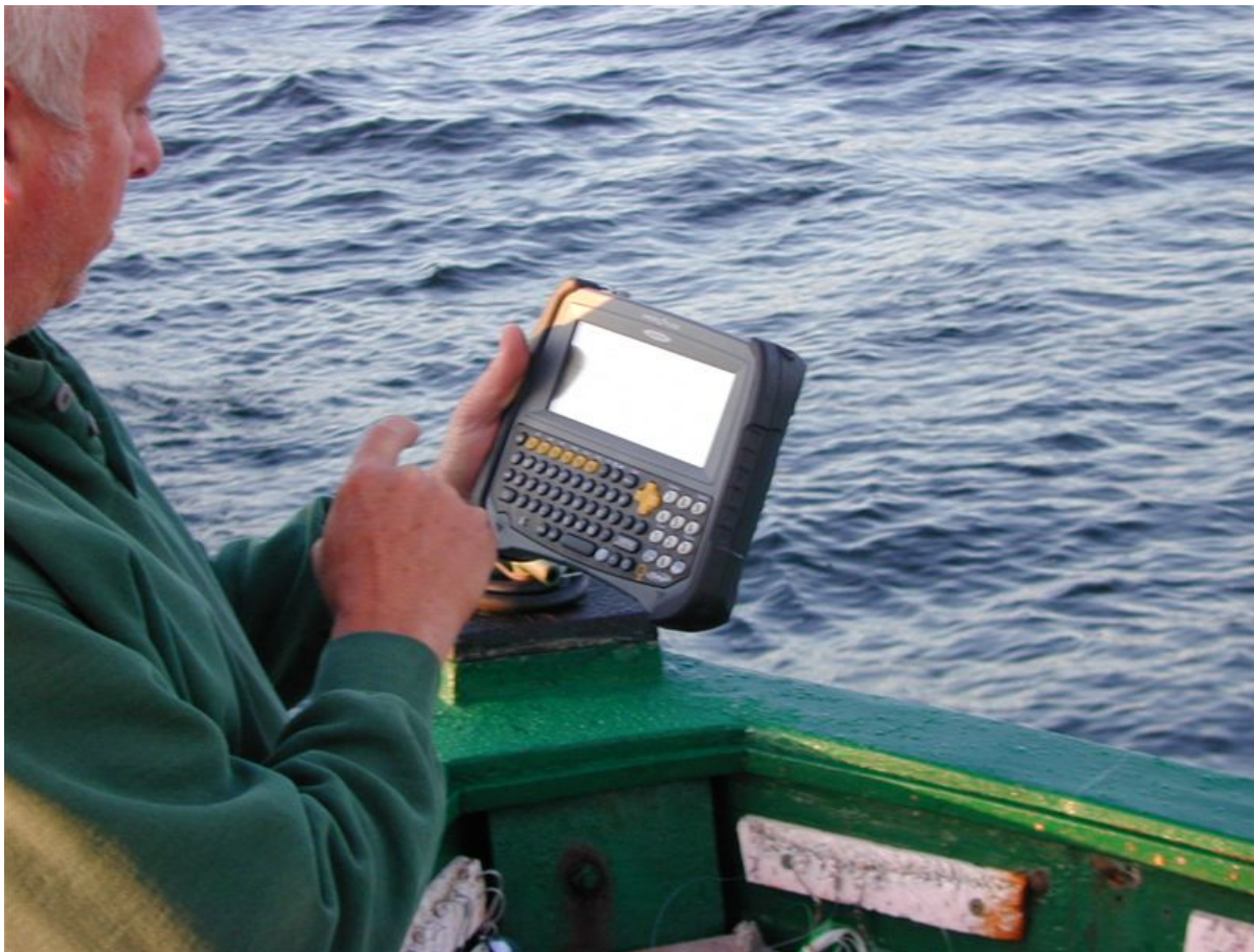
Figure 1. Commercial data entry system tested in 2006. The user interface is complex, screen has poor visibility, battery life is short, and per-unit cost is high. Subsequent developments have
