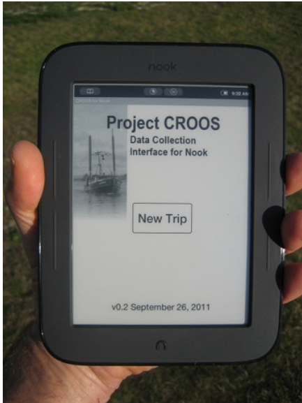
Figure 2. NOOK e-reader tablet showing visibility of E-Ink screen in full sunlight.
