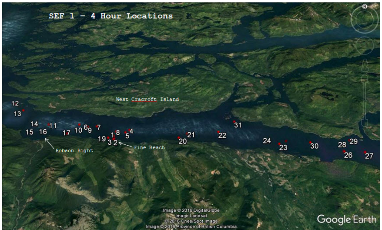
Figure 6. Illustration of the tracking data obtained by the surface current tracking technology (SCT) developed by IOS. This particular buoy was deployed 0.5 km east of Fine Beach on July 27 and stopped sending a signal 7 km northwest of Fine Beach on August 3.
