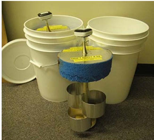
Figure 3. Surface current tracker shortly before deployment. To minimize the direct effects of weather on the SCT movement, the majority of the SCT floats below the surface with only the SPOT Trace above the water surface.
