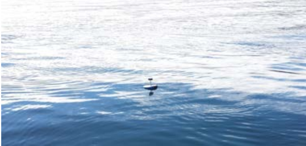
Figure 4. GPS surface current tracking buoy developed by the Institute of Ocean Sciences.
