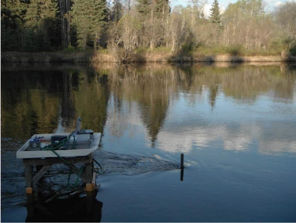
Figure 5. Photo of the hydroacoustic system collecting side-looking acoustic data from the river's left shore. May 25, 2014.
