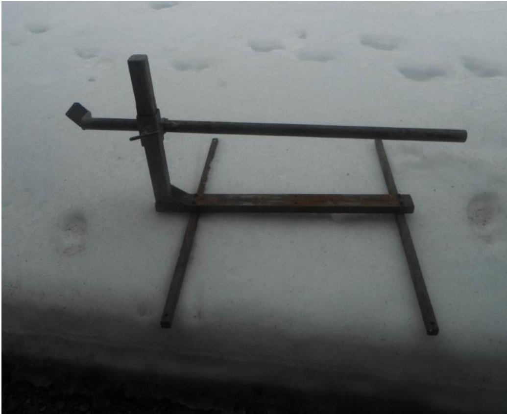
Figure 4. Photo of the steel structure designed and fabricated to mount the acoustic transducer horizontally.
