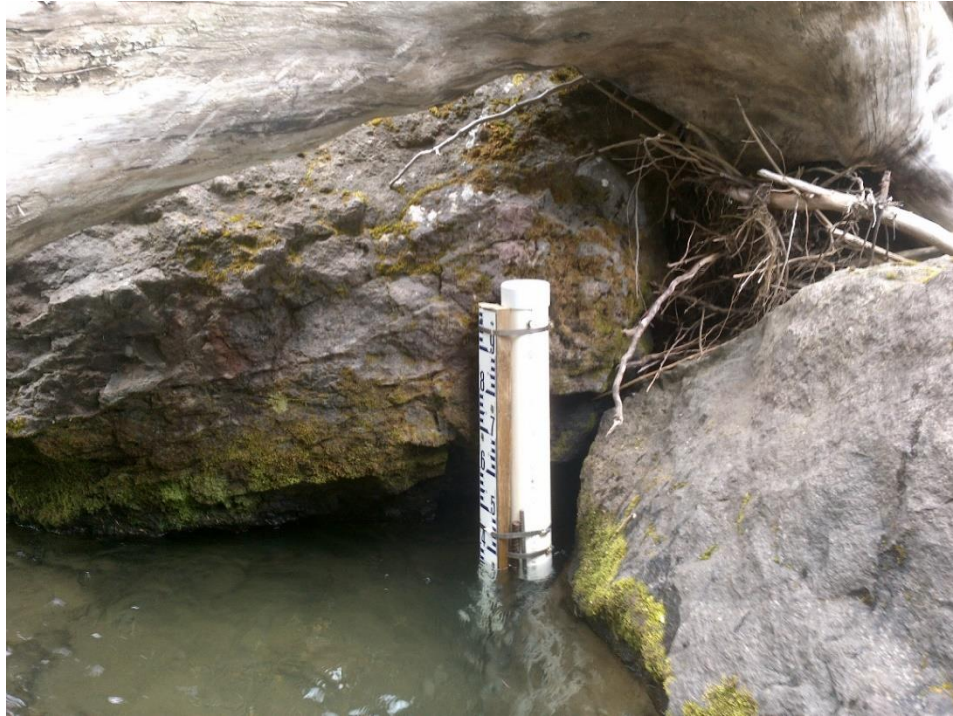
Photo 1: The hydrometric station as installed on July 30, 2016.
