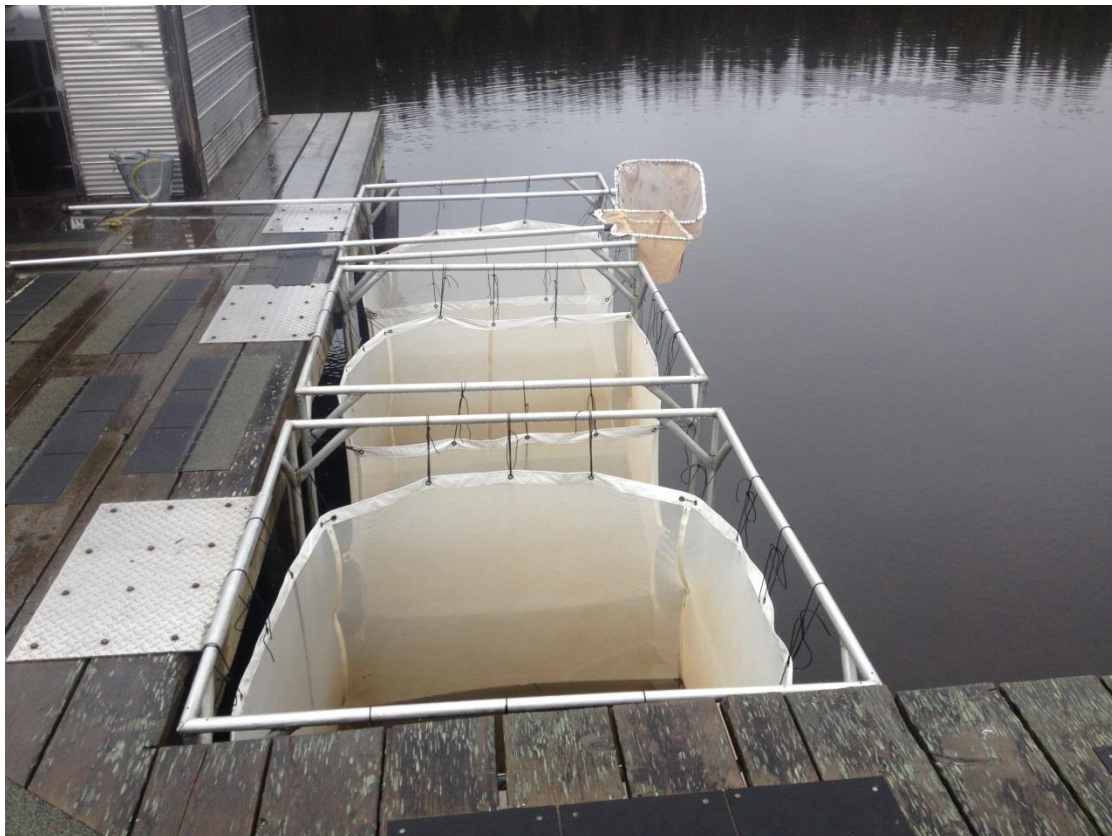
Figure 7. Three of five holding pens used to hold smolts until the smolts were enumerated and examined for tags.
