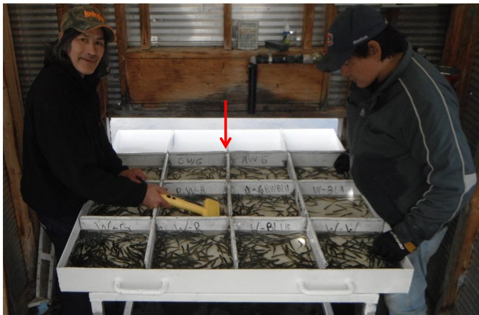
Figure 14. The yellow “T-Wand” coded-wire tag detector being used to locate live tagged smolts. Recaptured tagged smolts are removed and sorted according to tag colour. After examination, the unmarked live smolts are released downstream through the hatch (red arrow) by removing the compartment grid and lifting the back end the sorting tray by the two handles visible at the front of the tray. Photo modified from Doire and Macintyre (2016).
