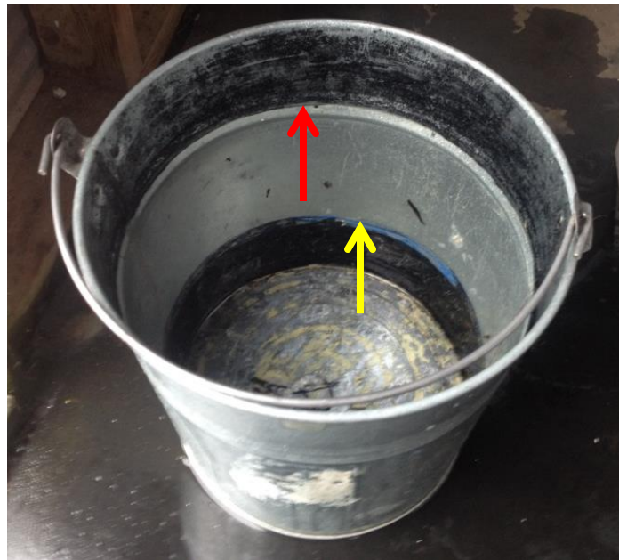
Figure 12. The volumetric “calibration” bucket used to quantify smolt numbers. The lower yellow arrow indicates the full mark to which water is added prior to filling with smolts. The upper red arrow indicates the level indicating the full mark to which smolts are added. As soon as the smolt “full” mark is reached, the live smolts/water mixture was immediately transferred to the counting shed ( Figure 14 ) where smolts were examined for tags.
